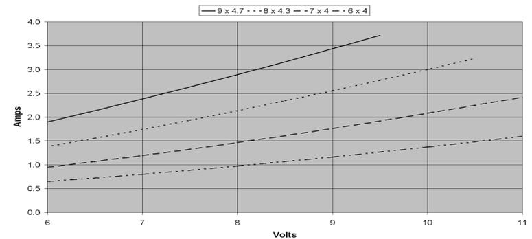
HC2208-1260 Current vs. Voltage with Propeller
