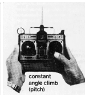
Climbing or descending is accomplished by constantly pressing the stick up or down.
