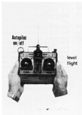
The AS-07 maintains level flight without any control input.
