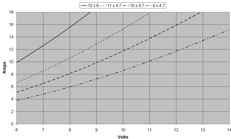
HC2816-1220 Current vs. Voltage with Propeller
