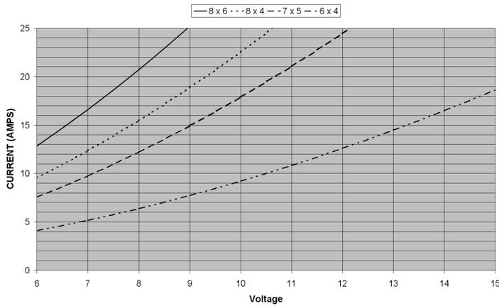
HB3615-2100 Current vs. Voltage with propeller
