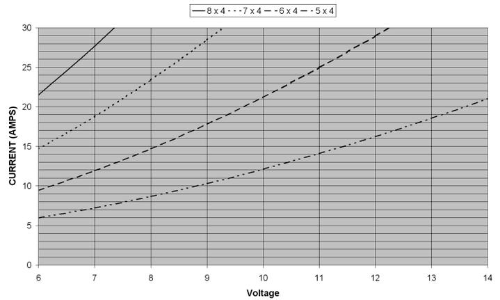
HB3615-3200 Current vs. Voltage with propeller
