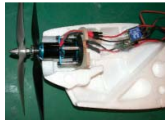
I installed the CRP in the Multiplex Acromaster by creating a 3/16-inch-thick firewall and gluing the new firewall deep inside the front of the model. I “potted” the firewall into place with a mixture of 5-minute epoxy and microballoons. You have to make holes for the two sets of ESC wires in the firewall in the upper left and the right sides. The supplied radial motor mount secures the motors to the airframe.
