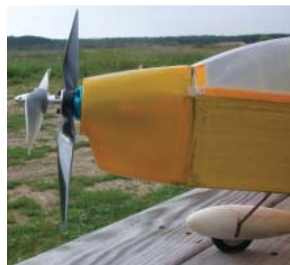
I installed the Himax CR2816 CRP drive system in an AeroCraft/Modelair-Tech T3D model. With the stock props, performance was exceptional at a burst power of 450 watts. When I replaced the stock 10x5 front prop with a 9x4.5, speed was a bit higher with a slight loss of static thrust.
