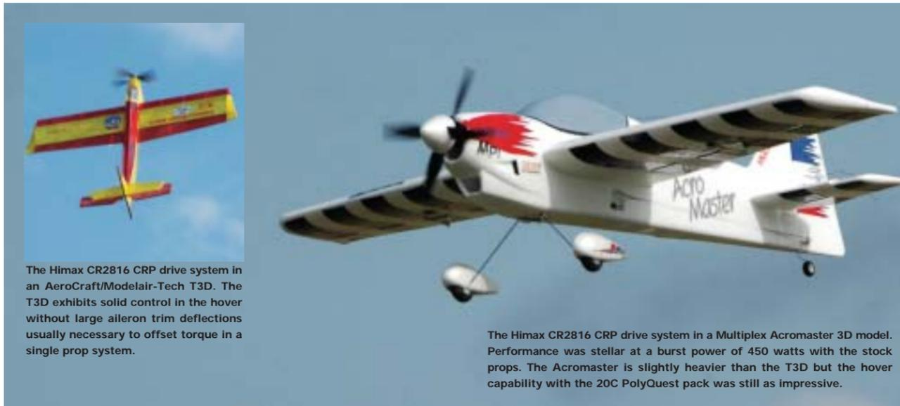
The Himax CR2816 CRP drive system in an AeroCraft/Modelair-Tech T3D. The T3D exhibits solid control in the hover without large aileron trim deflections usually necessary to offset torque in a single prop system.
