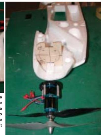
for the combined system at full throttle. This is 25 percent more power than specified by Himax for this system. I believe the discrepancy is the result of my using a battery with a much lower resistance than Himax used in their tests. If I used a much smaller pack, say a 2000 to 2200mAh pack, the power would easily drop to around 350 watts, as a pack of that size cannot sustain the same voltage level under load as
